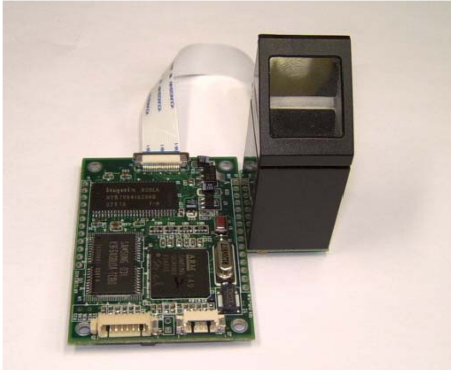
Picture 5. BKS-1700, Front : connecting optic scanner to board 1(BKS-1700)
