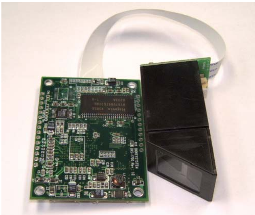
Picture 6. BKS-1700, Rear: connecting optic scanner to board 2(BKS-1700)
